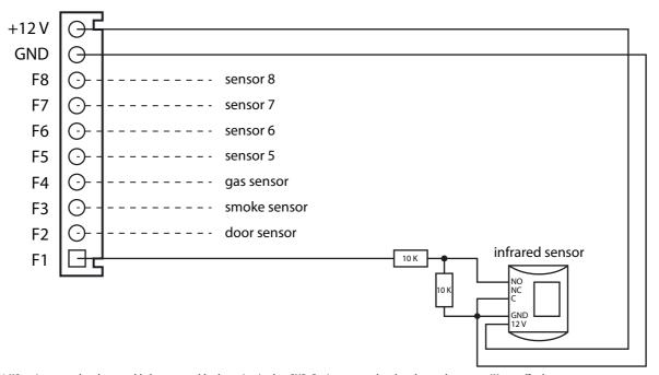
NOTE: 10 K $\Omega$  resistors used to detect cable by cut or cable short circuited to GND. Resistors must be placed near the sensor. IU can afford sensor 12 Vdc - 300 mA type.
